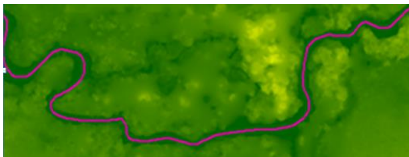
Fig. 3. The riverbed shown in the Digital Terrain Model (DTM) fragment (based on UAV data) coincides with the interpretation result – in 2022
