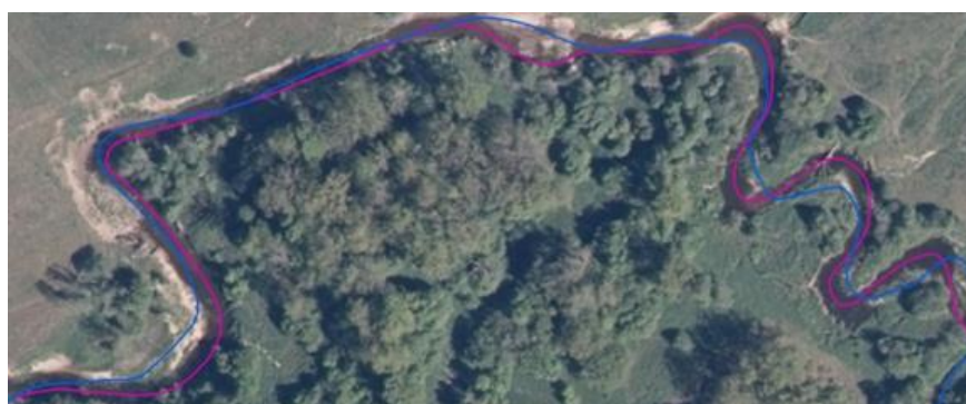
Fig. 2. Changes in the axial line of the river bed: GDR10LT data (blue) – in 2003; data compiled by drone (red) – in 2022
